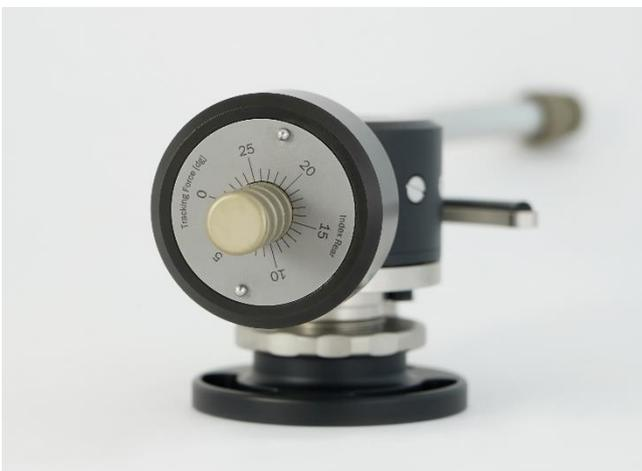
The counterweight is connected to the arm-tube by two decoupling PTFE bushings. It features a spring-loaded mechanism to allow backlash-free positioning along the adjustment range. An engraved scale can be turned to zero position when the tonearm is in neutral balance. This allows precise setting of the vertical tracking force, even if you don't have a tonearm scale at hand.
