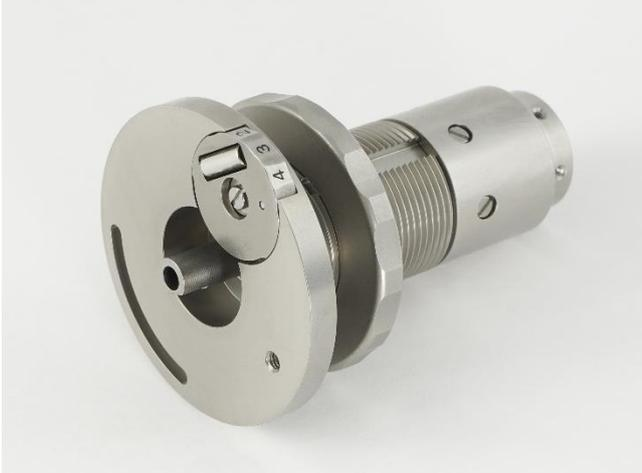
Each EMT tonearm consist of 150 individual parts. All structure parts are machined from solid material in highest precision. We use stainless steel for the base-parts and aluminium-alloy for all movable parts. A specific alloy called “German silver” is used for all parts that are exposed to mechanical abrasion, such as the rear shaft or the connection for the Tondose.
