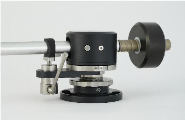
All tonearm models feature a magnetic anti-skating device and a ring for VTA adjustment. A tonearm-lift is included with the product and can be removed if the tonearm is used on old EMT turntables with built-in lifting device. The tracking geometry was optimized according to the latest knowledge, but all mounting properties remain unchanged.
